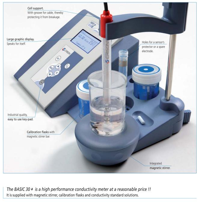
The incorporated electronics adapt to platinum and titanium cells. Titanium cells are highly recommended for dirty and viscous samples.
